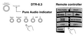
**Direct/Pure Audio:** Changes the listening mode for the signal type that is currently being input from the selected input source to the Direct listening mode. If pressed, the corresponding setting in the Listening Mode Preset Sub-menu of the Input Setup Menu for the selected input source is also changed. When the listening mode is set to Direct, you can switch between Direct and Pure Audio.
